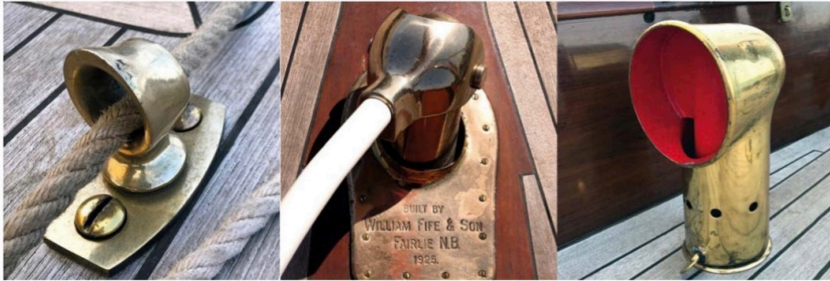
Above: Bonnet fairlead; Tiller stock with builder's plate; deck vent
